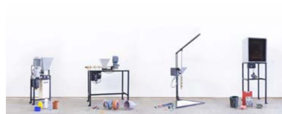
Exhibit 11: Precious Plastic's shredder, extruder, injection and compression machines 88
