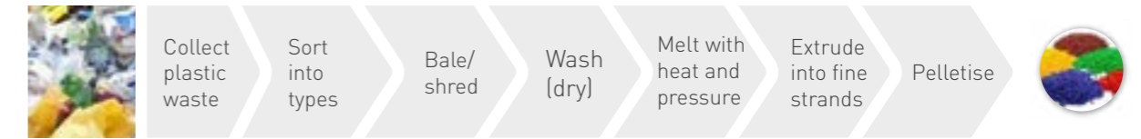
Exhibit 5: Processing steps to convert waste plastic into plastic pellets
